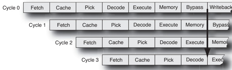
Figure 1.10 Pipelined instruction execution including bypassing of results
